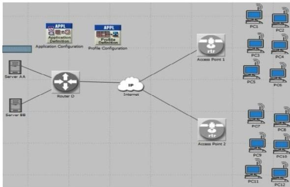
These access points are connected by PPP-DS1 to Router S connected by PPP-DS1 to IP cloud (Internet) connected by PPP-DS1 to Router D connected by PPP-DS1 to two Servers (Server AA, Server BB) which represents two departments.
